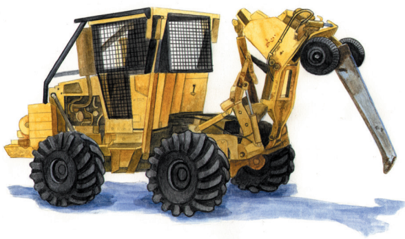
Figure 8.—A vibratory plow is sometimes used to disrupt grafted roots to prevent local spread of oak wilt.
